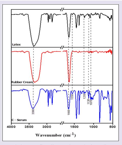
**Figure 4:** Absorbance spectra of latex, rubber cream and C-serum phase determined by Fourier Transform Infrared (FTIR).
