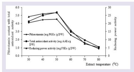
Figure 4: Effect of the temperature on extracted phlorotannin contentand antioxidant activities.
