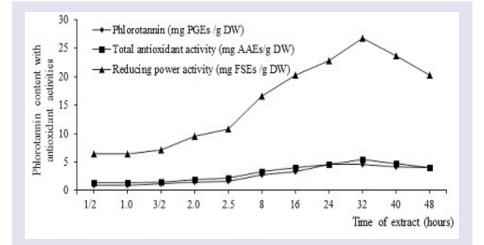
Figure 5: Effect of extracting time on extracted phlorotannin content and antioxidant activities.
